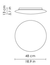
Wall/ceiling lights in satin finish triplex opal blown glass, with embossed aluminium internal reflector, and a chlorine-resistant, anti-UV, neutral translucent polycarbonate base. Twist-lock system for the glass component. The Bis collection has IP44 protection.
